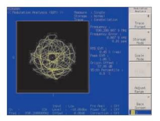
The following screen represents constellation display of the 8PSK modulation through Niquist filter and Gaussian inverse correction filter.
