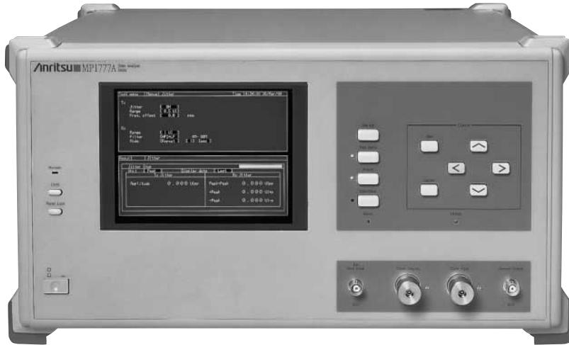
The MP1777A is a measurement solution for jitter evaluation. It supports both the STM-16/32/64 and OC-48/96/192 bit rates. In addition to supporting the bit rates of 2488.32, 4976.64, and 9953.28 MHz two additional bit rates used in submarine cable systems can be added as options.
