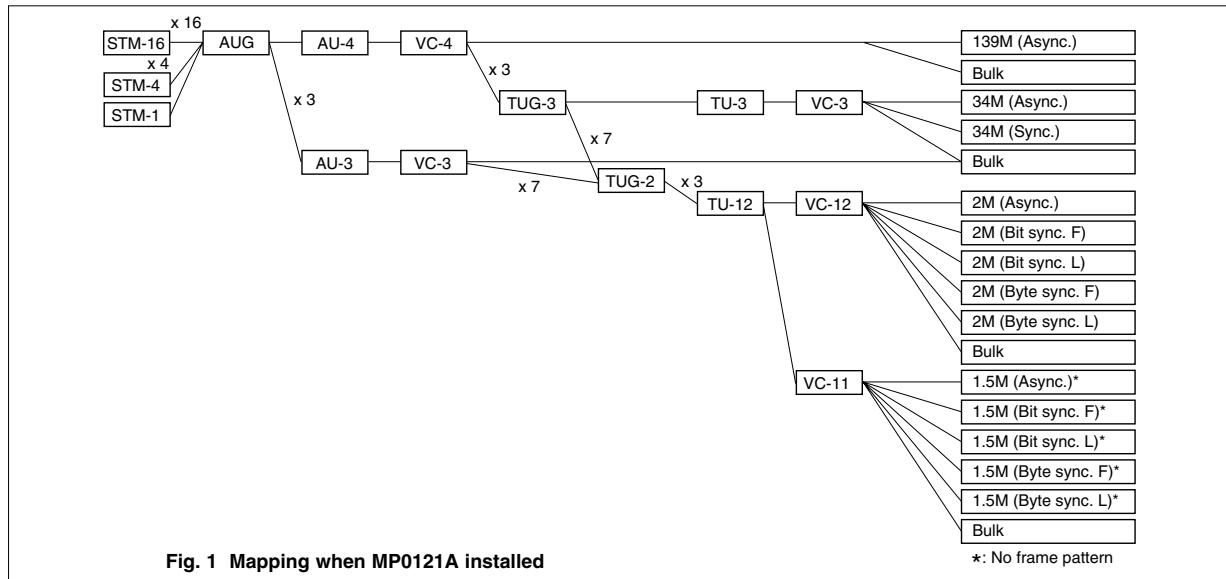
Fig. 1 Mapping when MP0121A installed
