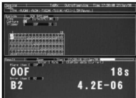
Measured errors/alarms can be displayed as a graph, and 1 second, 1 minute, 15 minutes, and 60 minutes can be set as the bar graph time units.
