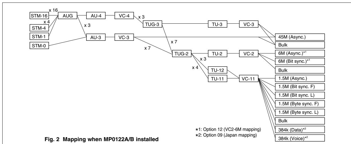
Fig. 2 Mapping when MP0122A/B installed
