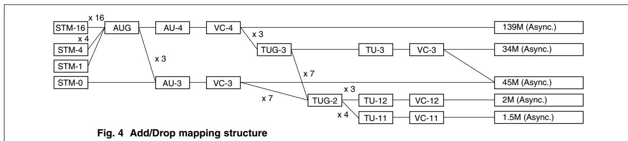
Fig. 4 Add/Drop mapping structure
