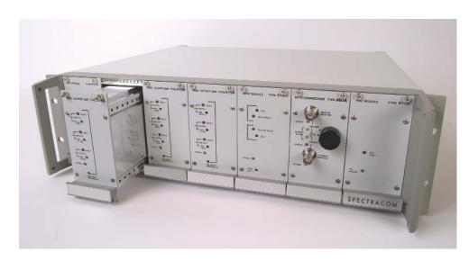
The 900-series distribution amplifiers are for local distribution of time code signals, 1PPS timing signals, sinewave reference frequency to multiple outputs, up to 30 per cabinet.
