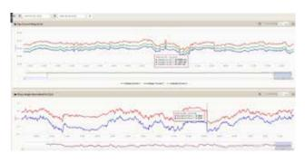
Data from three HV bushings on a 660 MVA GSU shows some rapid changes in current magnitude: up to 7% per hour may be seen and is normal at this location.
