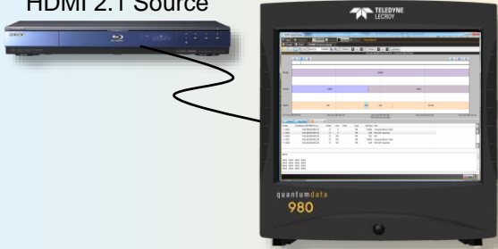
Test Setup for Source Test
