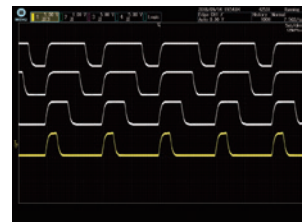
Using snapshots (white waveforms)
