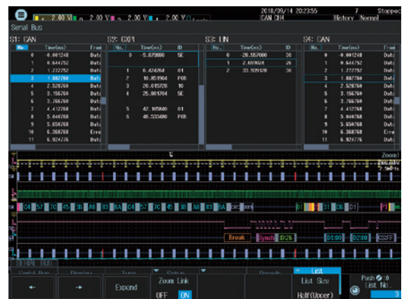
Four bus decode and list display
