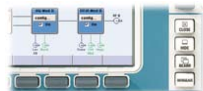
Softkeys and hardkeys of the R&S®SMU200A for windows management
