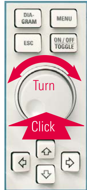
Rotary knob for navigation in the menus
